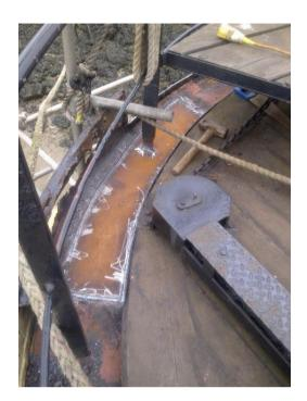
Finished scraping half the ship. Blow lamped, then painted one third of the bottom up to the top chine, see photo. Painted all of the port side from the bottom chine up to water line. Cut plate and fitted. Welded the repaired plate in the gutter, see photo. (Jason heated; Julian hit it until it fitted) Jason is a good welder, right up to the joins and rivets.
