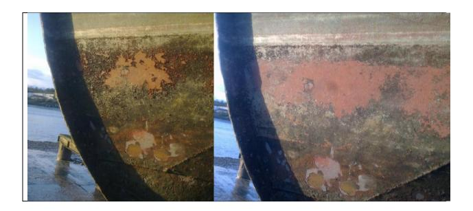
These are also two of the rudder pintle. We jacked the trailing edge of the rudder to move the pin and it moved between 4 to 6 mm sideways. Julian could get a piece of 3.5mm welding rod (flux cleaned off) down the gap to try to find the length of the pin which seems to be about 40 to 50mm into the socket. Photos show all the sideways movement, there is no up and down movement.
